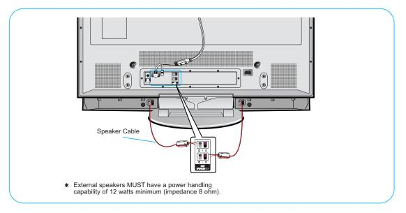
Connect the speaker audio cable to the external speaker output jack on the PDP matching the "+" and "-" ends of the cable with the diagram on the PDP.
